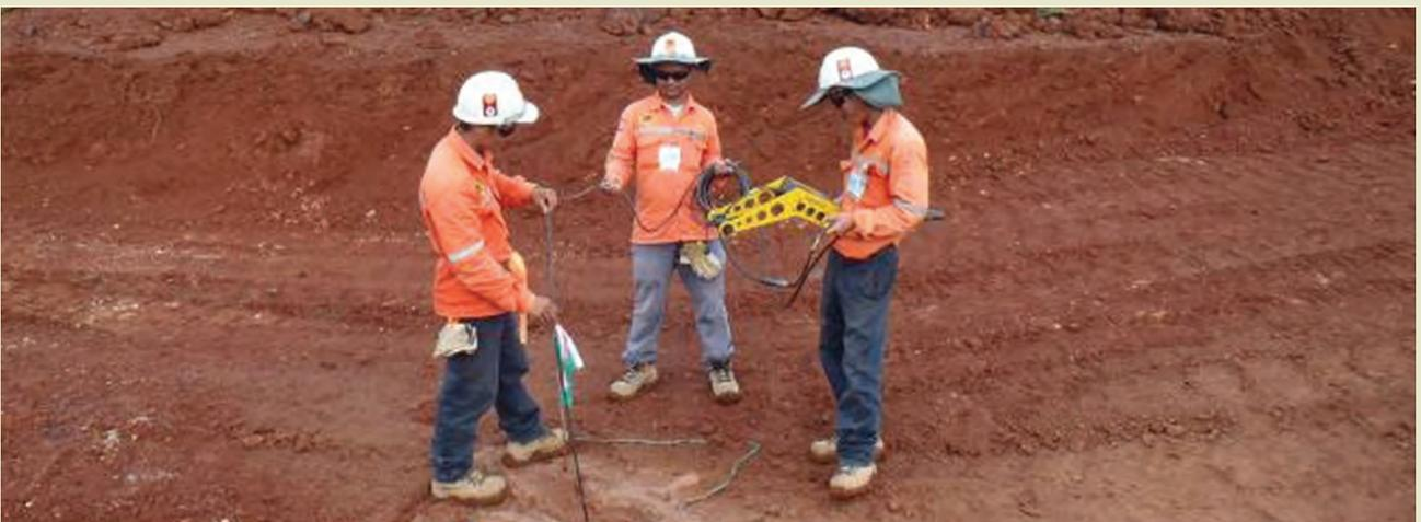
*Bore Hole Clearance using Foerster 4032 (Photo courtesy of the UXO Geophysics Cell)*
