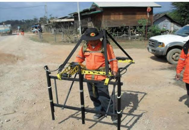
Foerster 4032 Triple Probe Setup for road clearance
