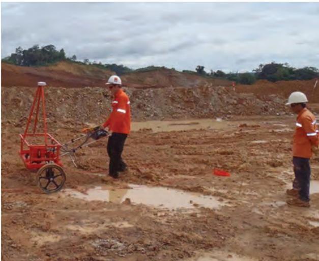
EM61 MK2A-HP being used to conduct clearance in a mining pit.
